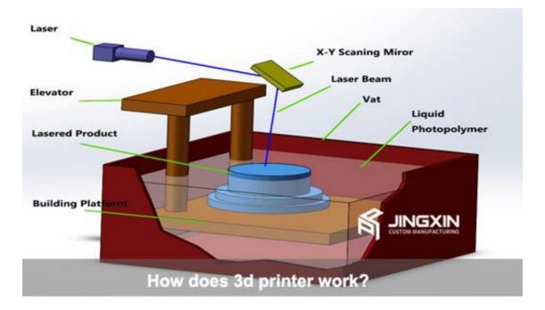
The advantages of light curing technology is that the molding speed is high, the prototype is high precision, and it is very suitable for the production of high precision and complicated structure parts. The use of light-curing technology for industrial-grade 3D printers, the most famous SLA 3D printer manufacturer is the Objet, They also offers more than 123 kinds of photographic materials, it is currently the most supportive material for 3D printing equipment.
