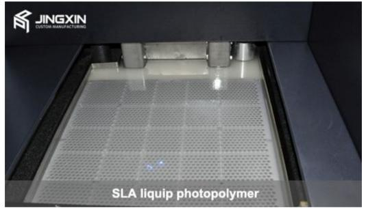
Light curing technology is the earliest developed rapid prototyping technology, is currently the most in-depth, the most mature technology, the most widely used one of the rapid prototyping technology. Light curing technology, the main use of photosensitive resin as the material, through the ultraviolet light or other light source solidification molding, layer by layer curing, and ultimately get a complete product.
